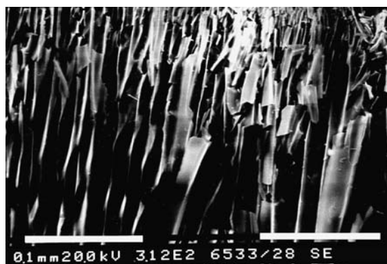
Figure 3. SEM picture of freeze-dried alumina-zirconia gel (sample A).
